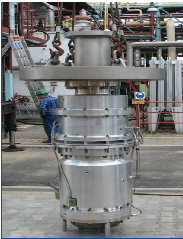
Figure 1. Upward flow two phase cryogenic liquid expander as delivered to Polish Oil and Gas, 2003.
