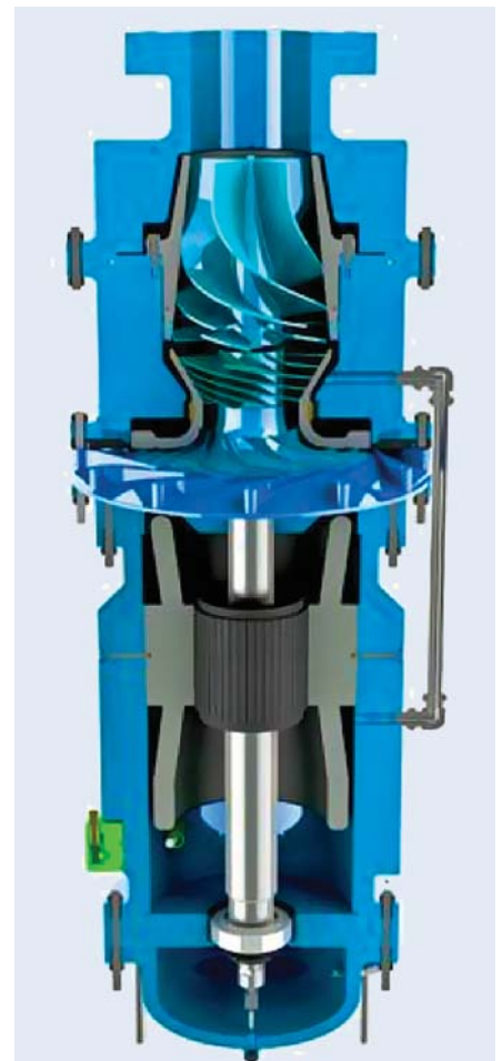
FIG. 9 Cross-section of a two-phase expander assembly.
