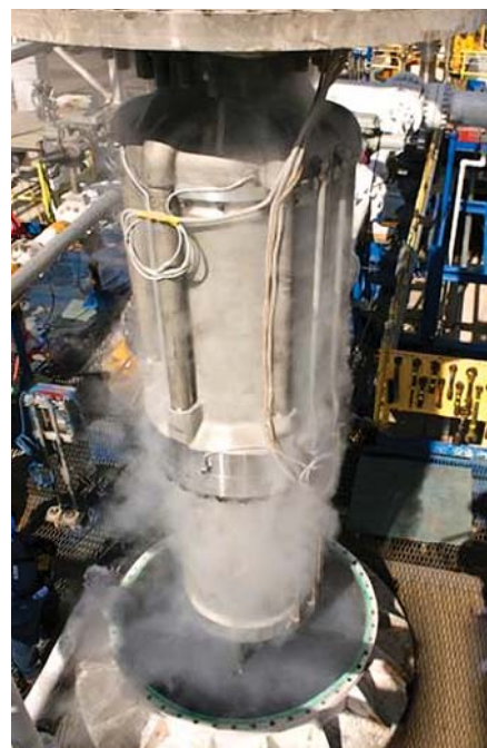
FIG. 2 An LNG sendout pump upon removal from a performance test stand.
